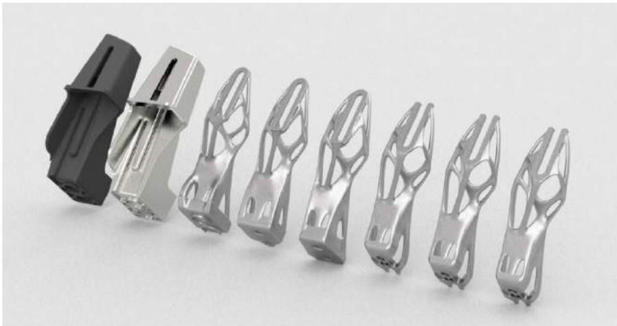
BMW's 3D printed roof bracket for the i8 Roadster (Source: Additive Manufacturing Today)
